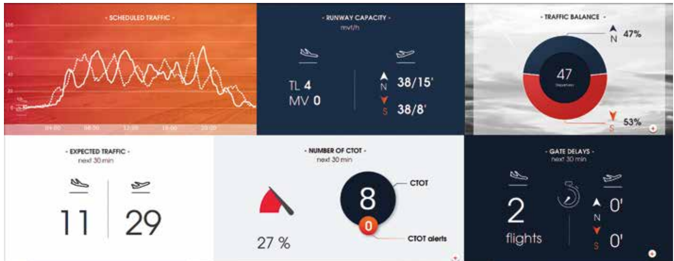
BigSky, a multi-service MMI for flight management in TMA and at the airport. In June 2019, Paris-CDG air traffic control services designed and introduced this tool with its groundbreaking MMI, presenting a set of ATFCM and CDM services on a single screen. Connected to the B2B@NM and to the airport data, this tool facilitates decision-making for the management of arrival and departure flows, the balanced use of the four runways, operations during traffic peaks...
