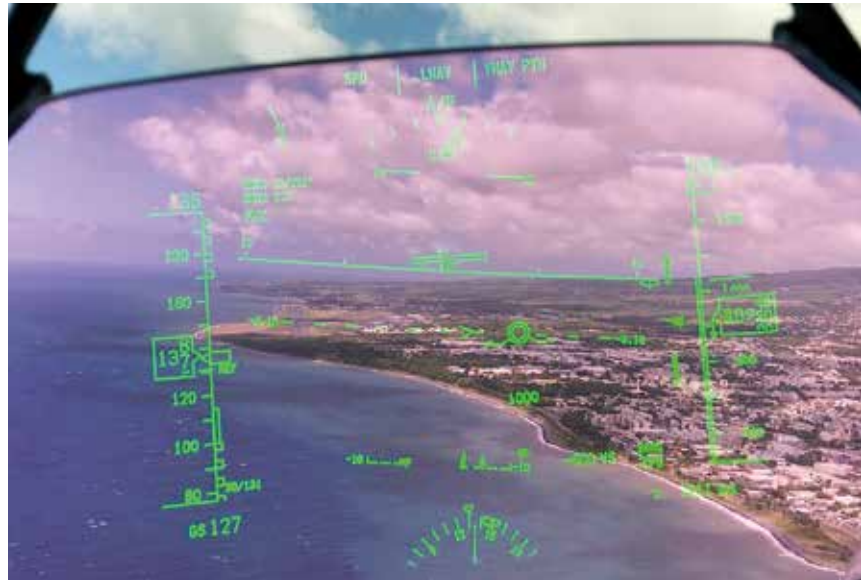
Saint-Denis de La Réunion: the DSNA in collaboration with Air Austral designed an AR RNP procedure on runway 12 that, in bad weather, provides a precision approach on the longest runway, used for take-offs and with no ILS. An important asset for flight operation and safety!
