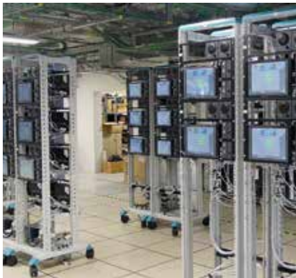
N-VCS project: DTI endurance tests on several operator positions.
