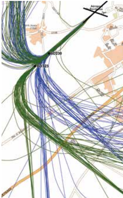
Saint-Denis de La Réunion: the DSNA in collaboration with Air Austral designed an AR RNP procedure on runway 12 that, in bad weather, provides a precision approach on the longest runway, used for take-offs and with no ILS. An important asset for flight operation and safety!
