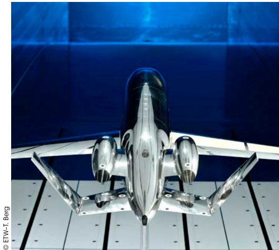
BUSINESS JET PROJECT: Falcon LSBJ (Low Sweep Bizjet Concept) from Dassault Aviation, with twin tail assembly, for masking engine noise groundwards.
