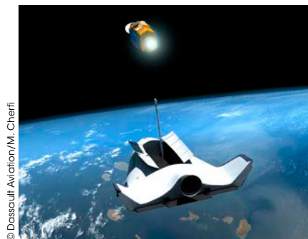
UNMANNED SUBORBITAL AIRCRAFT: Dassault Aviation "VEHRA" launching a satellite into low orbit.
