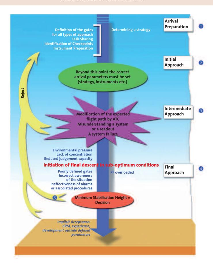
The unstabilised approach can be described by a chronological chain of individual factors which can interfere with the crew's management of the flight (see diagram). There are two critical phases of note: the final segment, during which the aircraft closes with the ground with reduced obstacle clearance margins; and the go-around, which although it is a segment entirely separate from the approach, is not necessarily executed under conditions foreseen by the procedure designer.
