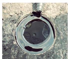
The product of a collaboration with the HiKoB start-up, this innovative system allows real-time information gathering on climatic developments on the road network. Thus winter road interventions can be initiated with optimal efficiency.
