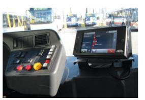
Navinéo is a system for real-time monitoring of a bus fleet using geolocalisation. The Engie Ineo firm has developed a variety of services: bus regulation, information on waiting times, incident management and requests for traffic light priority.
