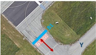
For a take-off on runway 22, GROUND controller tells the pilot to taxi and hold short of holding point B1. When the pilot approaches B1, GROUND controller transfers him to the tower frequency. Watchfulness is particularly required for this short taxiway because there is no Wig-Wag unlike B5, and depending on time of the day, glare can interfere with pilot's vision.
