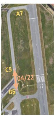
When vacating the runway 17/35 on A7, the pilot must remain on tower frequency, because to taxi to apron, runway 04/22 has to be crossed. This crossing is done in two ways depending on traffic:
