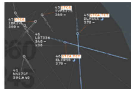
The safety net for en-route (STCA) alerts the controller when aircraft in flight are in hazardous proximity to dangers.
