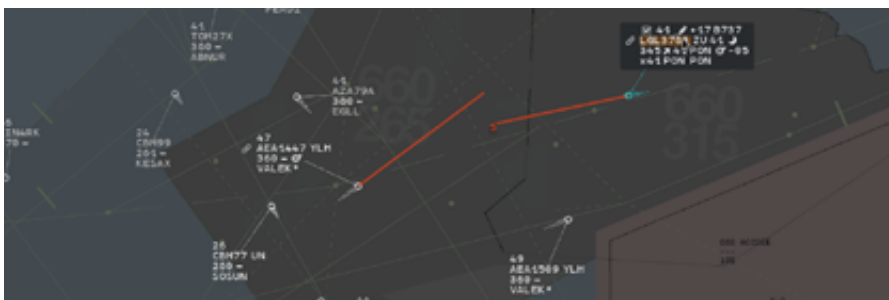
The Tactical Control Tool (TCT) prevents controllers from potentially serious operational situations. If the controller types in conflictual clearance information, the TCT sends them an alert.
